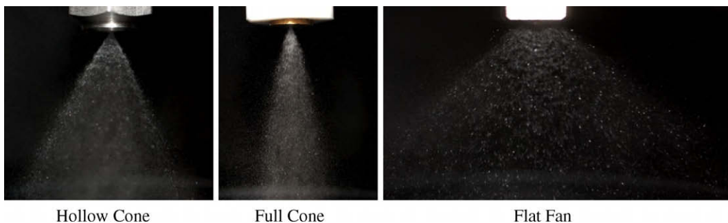
Fig. 2. Photographs of sprays produced by three nozzle types operating at 344 kPa.
